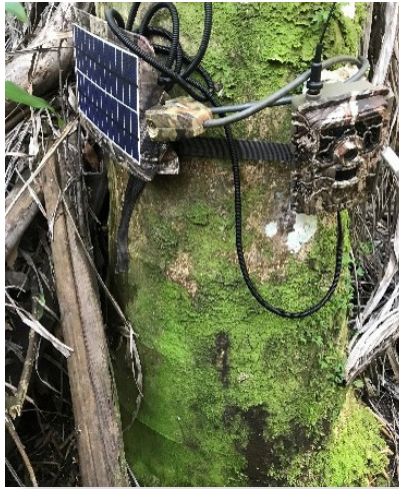
Cellular trail camera setup with solar panel.
